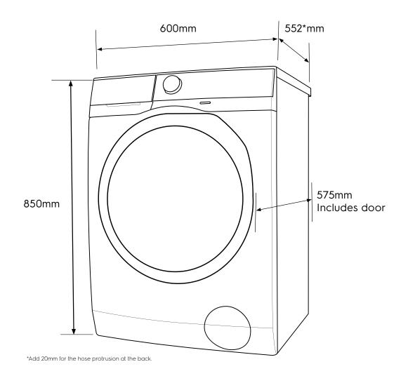
Please note! Dimensions to be used as a guide only. All customers MUST refer to the user manual supplied with the product for detailed installation instructions. © 2021 Electrolux S.E.A PTE. LTD. E\_DIM\_EWF8024P5WB\_Jun21
