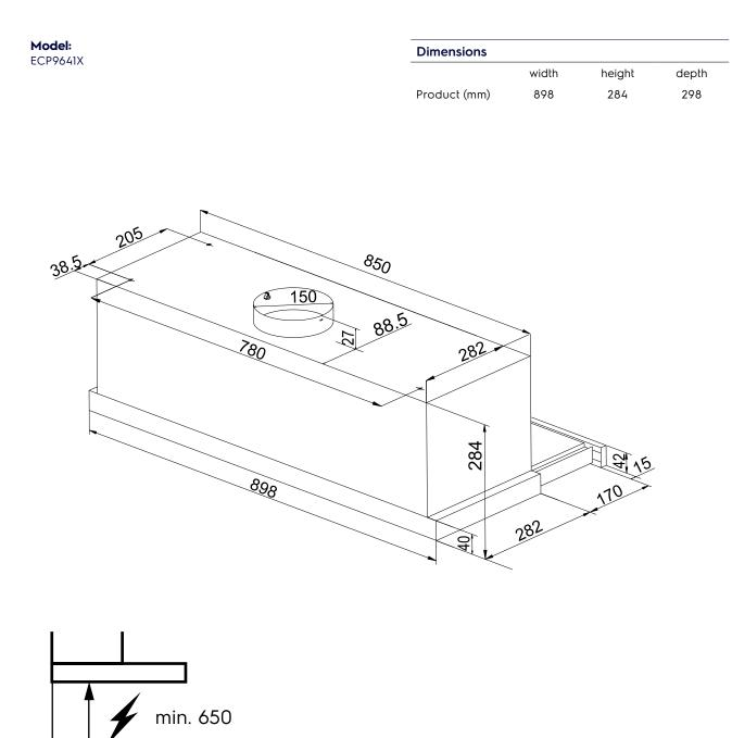
Please note! Dimensions to be used as a guide only. All customers MUST refer to the user manual supplied with the product for detailed installation instructions. © 2022 Electrolux S.E.A PTE. LTD. E\_DIM\_ECP9641X\_Mar22
